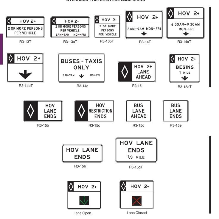
A lane-use control signal may be incorporated into an overhead preferential lane regulatory sign to indicate the status of a reversible operation as shown in the following example:
