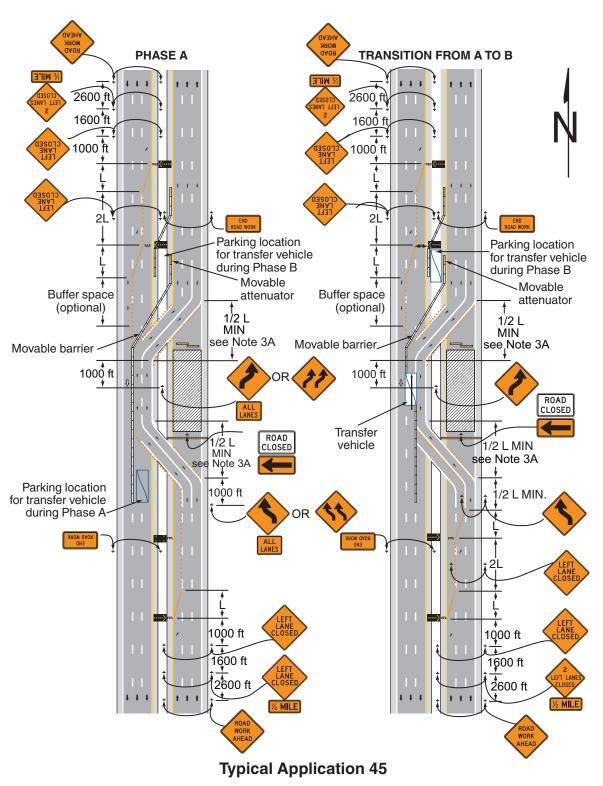
Note: See Tables 6H-2, 6H-3 and 6H-4 for the meaning of the symbols and/or letter codes used in this figure. Although leader lines point to the signs on the right-hand side of the roadway, most of these signs should be installed on both sides of the roadway.
