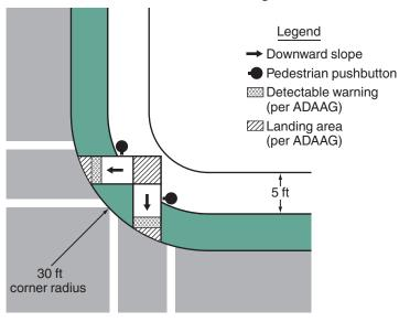
F - Perpendicular ramps with sidewalk set back from road with crosswalks far apart
