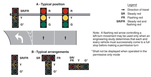
is required in order to provide a three-section signal face, but shall not be displayed during the permissive only mode.
