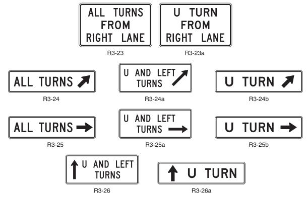
Figure 2B-8 shows the various signs that can be used for signing jughandle turns. Figure 2B-9 shows examples of regulatory and destination guide signing for various types of jughandle turns.
