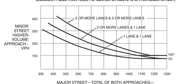
\*Note: 100 vph applies as the lower threshold volume for a minor-street approach with two or more lanes and 75 vph applies as the lower threshold volume for a minor-street approach with one lane.
