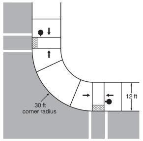
**B** - Parallel ramps with narrow sidewalk
