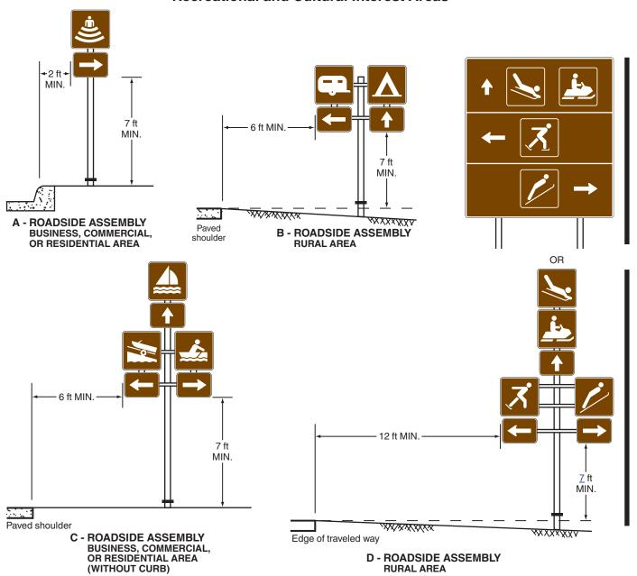
Note: See Section 2A.19 for reduced lateral offset distances that may be used in areas where lateral offsets are limited, and in urban areas where sidewalk width is limited or where existing poles are close to the curb.
