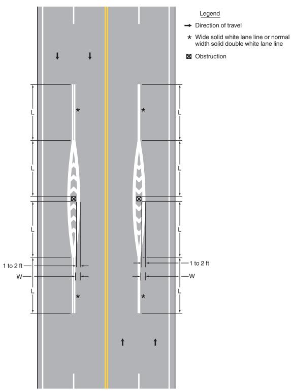
For speeds of 45 mph or more: L = WSFor speeds of less than 45 mph:  $L = WS^2/60$ S = Posted, 85th-percentile, or statutory speed in mph W = Offset distance in feet Minimum length of: L = 100 feet in urban areas L = 200 feet in rural areas
