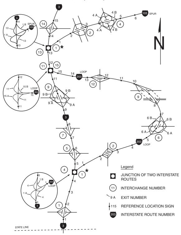
★ The freeway/freeway interchange where the beginning of the loop or spur route intersects with the mainline route may be called either Exit 1 or Exit 0 on the loop or spur route.
