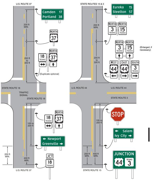
Note: The spacings shown on this figure are for rural intersections. See Sections 2D.29, 2D.30, 2D.32, 2D.34, 2D.40, and 2D.42 for low-speed and/or urban conditions.
