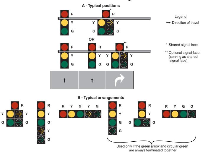
RED ARROW signal indication) or a steady CIRCULAR RED signal indication shall be displayed if it is intended that right turns on red be permitted.
