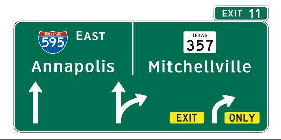
Where used, the Overhead Arrow-per-Lane guide sign at the exit or split shall be located at or in the immediate vicinity of the point where the exiting lanes begin to diverge from the through lanes or, for a split, at the point where the approach lanes begin to diverge from one another, preserving the relation of the arrows displayed on the sign to their respective lanes. The Overhead Arrow-per-Lane guide sign at the exit shall not be located at or near the theoretical gore.
