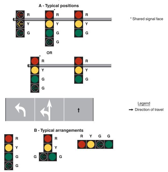
Note: Shared signal faces shall only be used for a protected-only mode left turn if the circular green and green left-turn arrow indications always begin and terminate together
