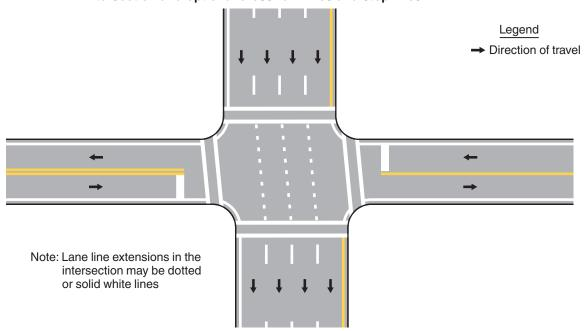
B - Typical pavement markings with double-turn lanes, lane-use turn arrows, and optional crosswalk lines, stop lines, and line extensions into intersection for double turns
