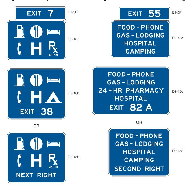
the service signing shall be repeated in smaller size at the intersection of the exit ramp and the crossroad. Such service signs shall use arrows to indicate the direction to the services.
