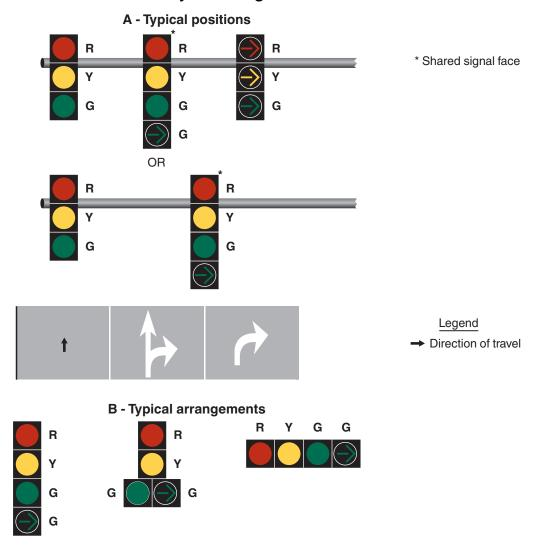
Note: Shared signal faces shall only be used for a protected-only mode right turn if the circular green and green right-turn arrow indications always begin and terminate together
