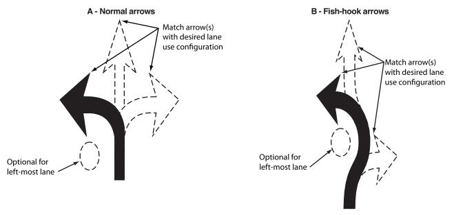
Figure 3C-3. Example of Markings for a One-Lane Roundabout
